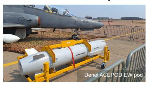
Weighing 326 kilograms and stretching over three and a half meters in length, it is the heaviest payload ever integrated onto a South African Hawk. The limited ground clearance of the Hawk's relatively low undercarriage posed additional challenges. To tackle this, the CSIR developed a custom trolley to safely load and mount the pod under the aircraft's center pylon.
