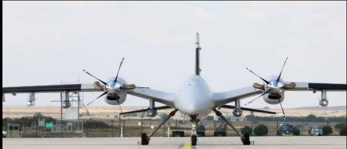
Combat drone Akıncı is seen loaded with domestic ammunitions in this screen grab from a video shared on Aug. 22, 2022. The combat drone, which is able to conduct flights with several ammunitions, bears domestically-developed ammunitions Teber-82 and mini munition MAM-T, together with mini munitions MAM-L and MAM-C on a multiple launcher station and the HGK-82 on the medium weapon station.
