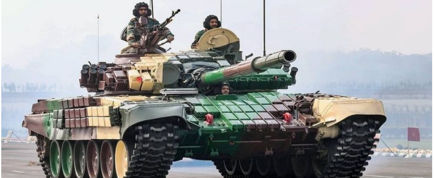
Ajeya MK1 (Unconquerable) – Indian version of the T-72M1. In parallel with buying various T-72M off the-shelf from the Soviet Union, India also launched its domestic production at Heavy Vehicles Factory. Ajeya MK2 – Indian version of the T-72M1 with ERA and banks of 6 smoke grenade-launchers on each side.
