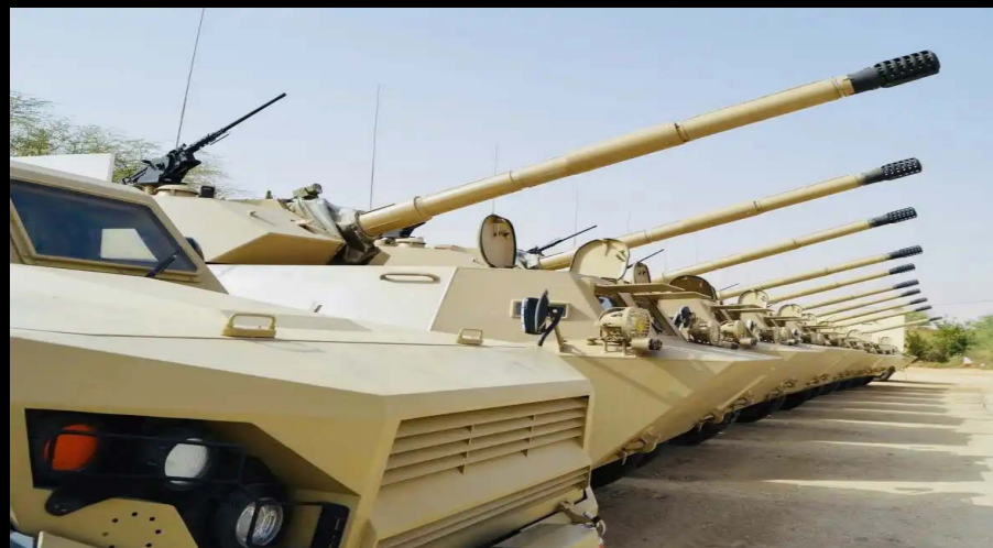
The WMA301 fire support vehicle, a Chinese export built on the 6x6 chassis of the widely utilized WZ551 Armored Personnel Carrier
