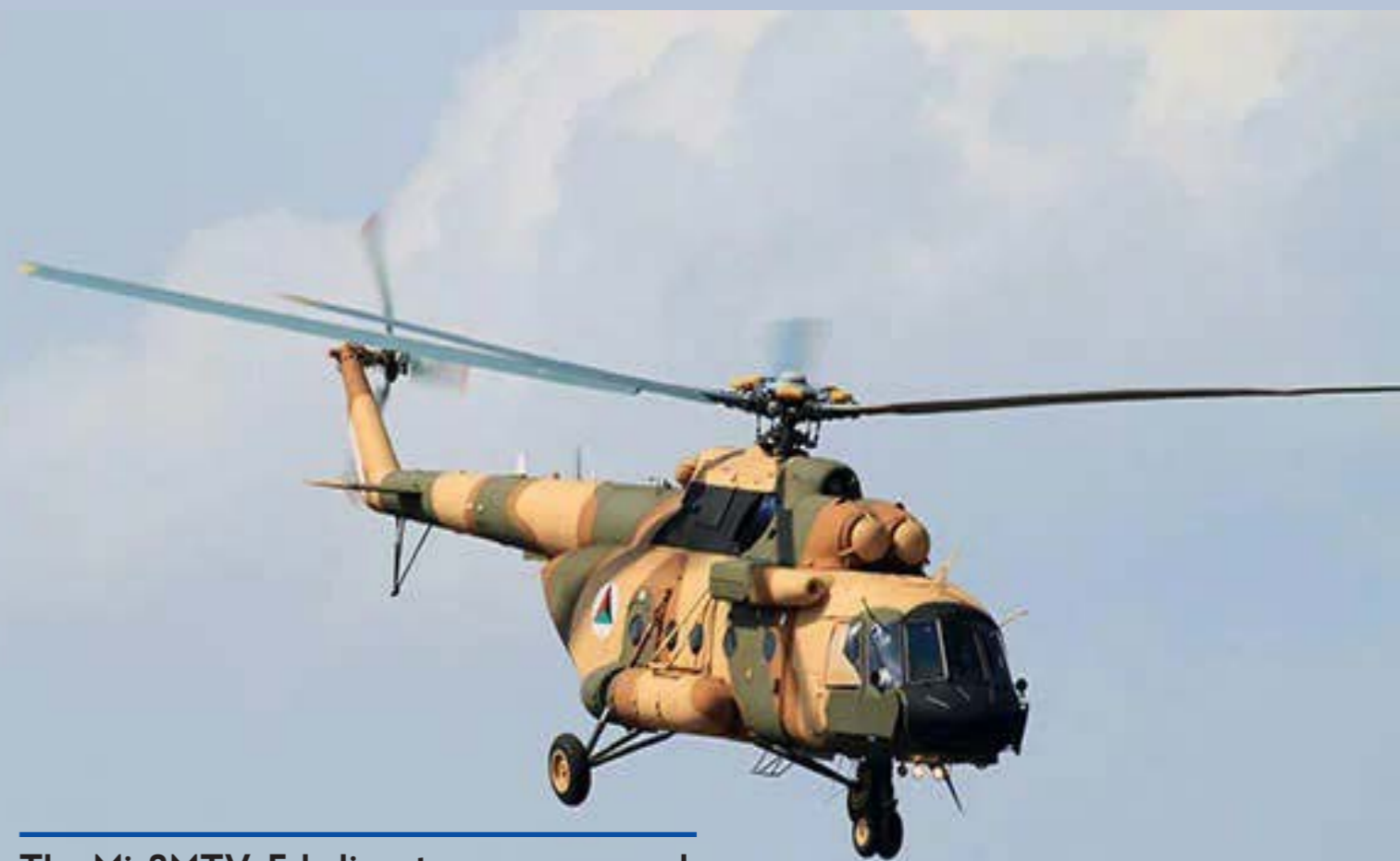
The Mi-8MTV-5 helicopters are powered by either TV3-117VM or VK-2500 engines. Image courtesy of Russian helicopters, JSC.
