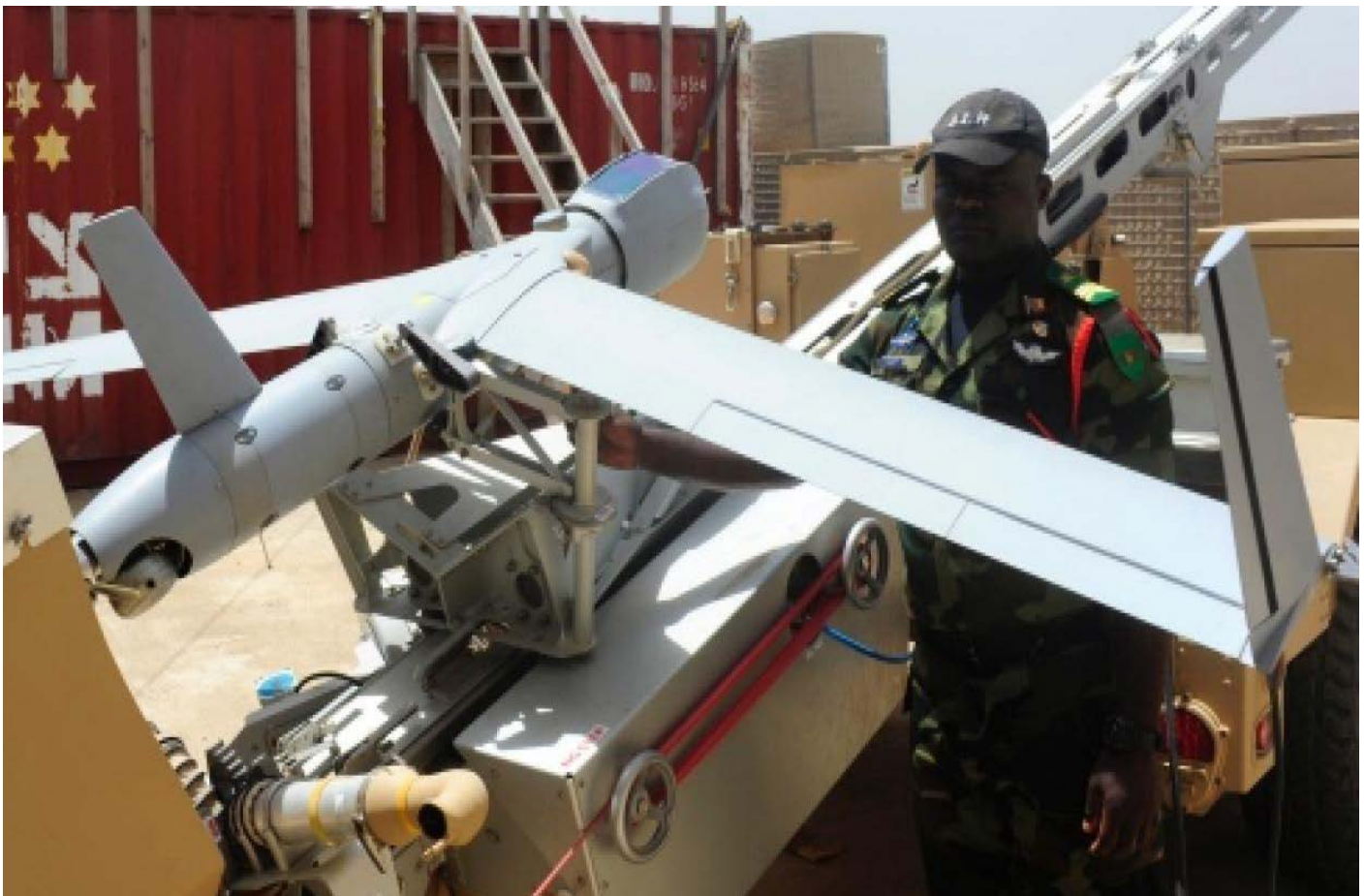
Boeing Insitu Scan Eagle Mini-UAS in service with the Cameroon military's special forces unit (BIR) (Credit: X)
